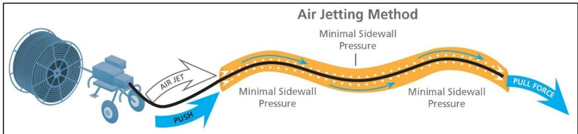
**Figure 6: Typical Air-assisted Jetting Method (not to scale)**
